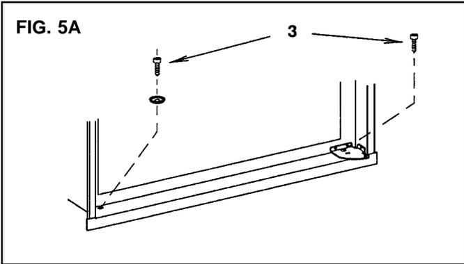
**b. Second: Install the two screws in the top frame.**
