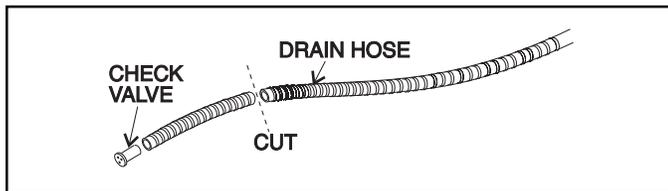
**NOTE:** Black water check valve must be reinstalled to ensure proper refrigerator operation. **DO NOT KINK HOSE.**
