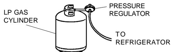
When testing the gas supply system at test pressures in excess of 1/2 psig, the refrigerator and its individual shutoff valve must be disconnected from the gas supply piping system.
