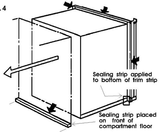
**NOTE:** Be careful not to damage the sealing strip applied to the floor of the enclosure when the refrigerator is put in place.
