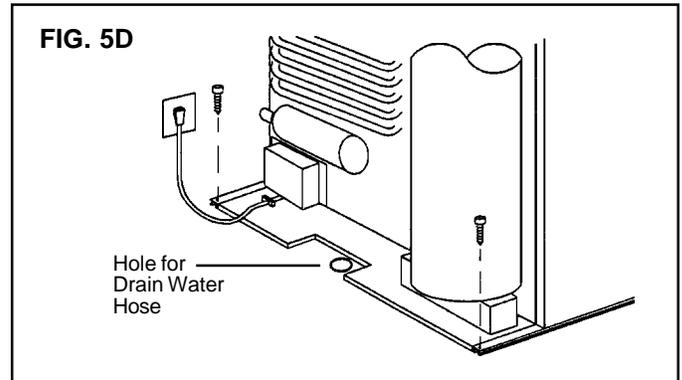
Failure to follow the sequence in securing the refrigerator in the enclosure can cause leakage between the frame and cabinet.
